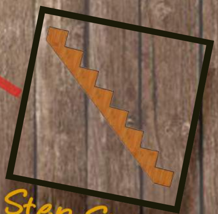
6 Step Stringer Overall Height: 48" Overall Length: 54"
