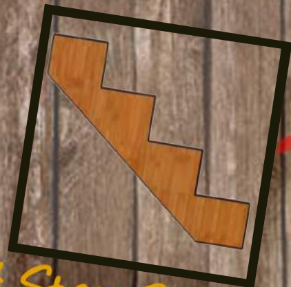
2 Step Stringer Overall Height: 16" Overall Length: 18"
